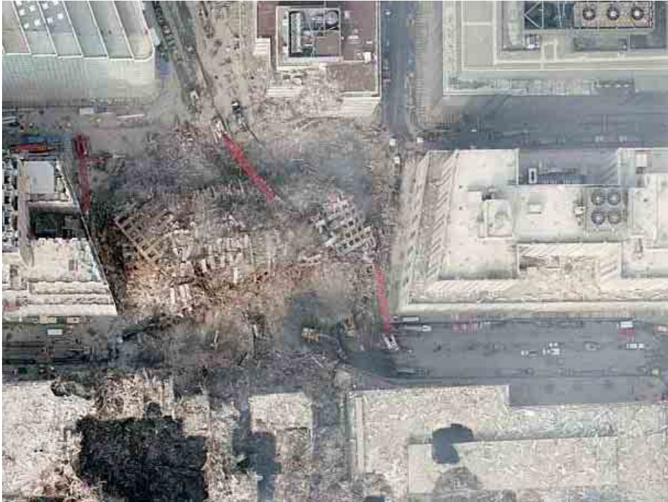
Figure 82. Debris from WTC7 did not reach the sidewalk adjacent to the Postal Building. (post 9/11/01) Source: http://forums.therandirhodesshow.com/index.php?act=Attach&type=post&id=19357
