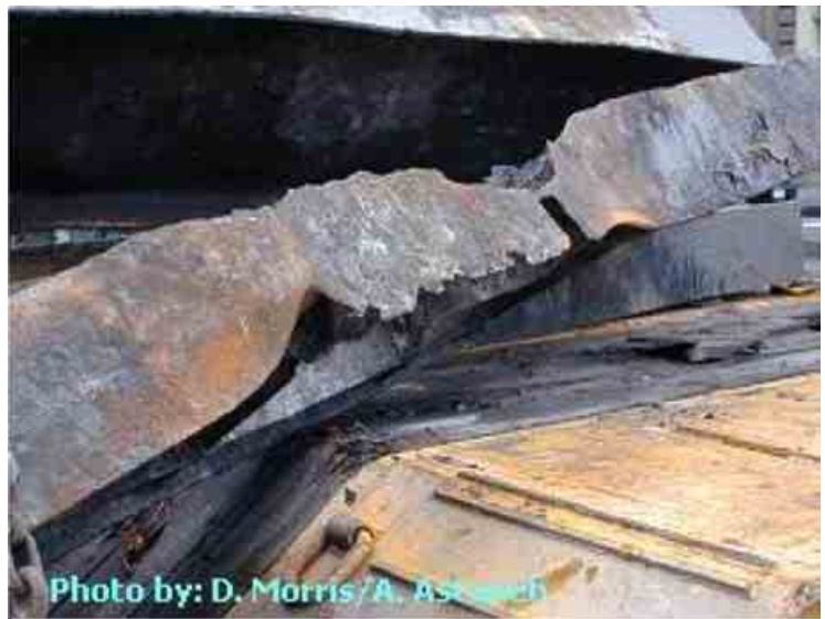
Figure 77. "A Beam Removed From the World Trade Center the Site Most Probably From Building 7" (Ref: Astaneh-Asl, 2002b) Source: http://www.nistreview.org/WTC-ASTANEH.pdf
