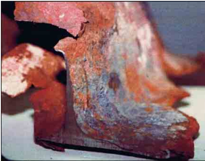
Figure 74. This piece of steel thought to be from WTC7 appears partially disintegrated. (Figure C-2. Closeup view of eroded wide-flange beam section.) (2002) Source: http://www.fema.gov/pdf/library/fema403_apc.pdf
