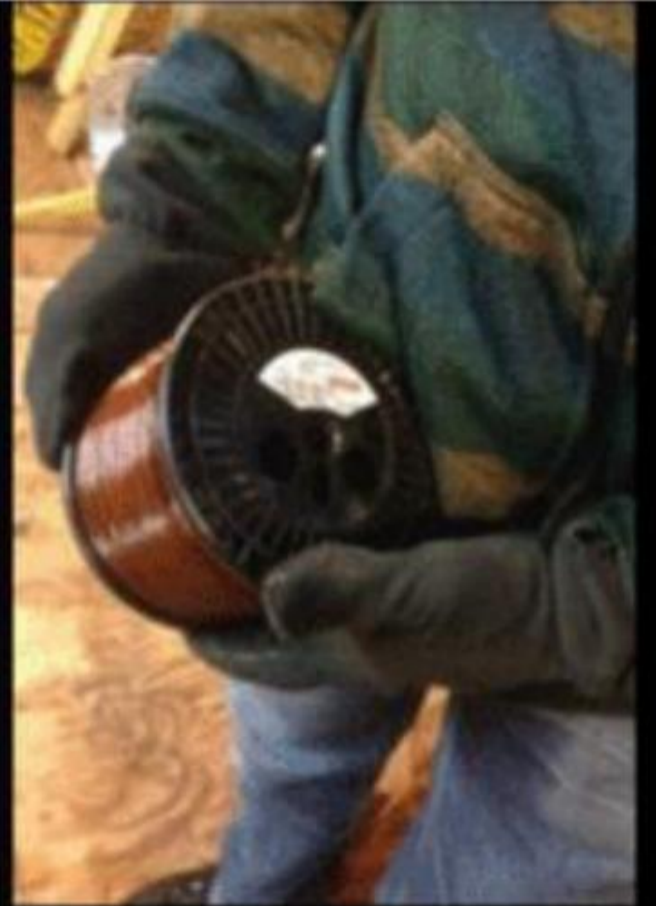
20 GAUGE MAGNET WIRE
