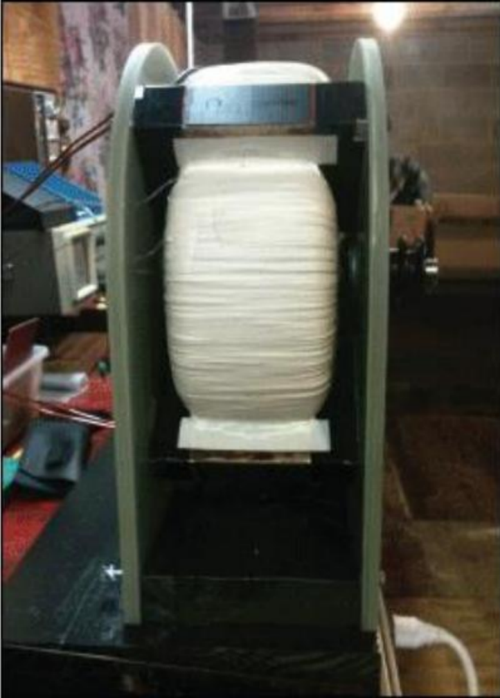
WRAPPED CORE/END PLATES
