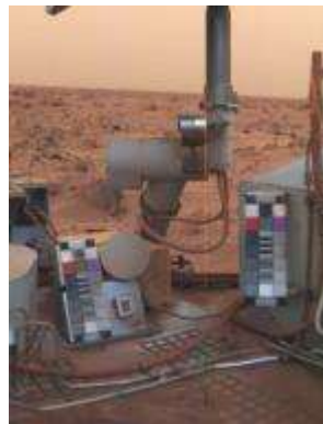
Photo of Lander’s top – showing the Camera Test Target (Viking image 12e018)
